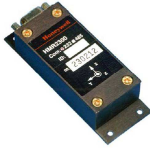
Figure 3.1: Photo of the Honeywell HMR 2300 as packaged for research personal computer. LabVIEW ® was used to collect the magnetic field intensity data and Matlab ® was used to complete all data processing in a post-processing mode.
