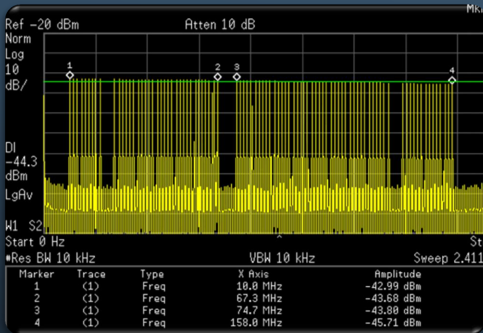
Spectrum analyzer capture of MCWB signal 550-700 MHz. 100 carriers
