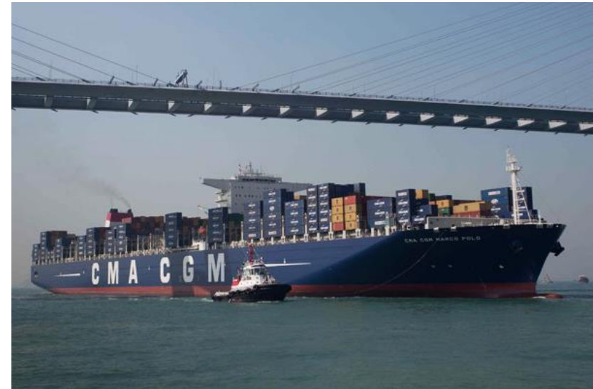
Container ship "Marco Polo", carries 16,000 containers, Asia - Europe, length 396 m, width 54 m
